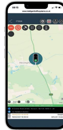
Example: showing a live 2Way mirroring what the traffic lights are doing on site. ITS54 on green and ITS53 on red.
