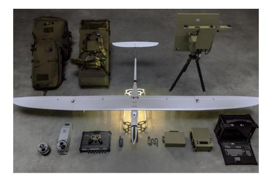
The observation head with two cameras (visible light and IR) attached under the fuselage of the FLYEYE mini UAV provides significantly better observation options and a function for rapid switching between the two video feeds.
