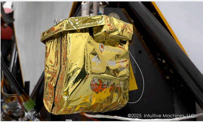
A deployer jointly developed with partners for transporting YAOKI to the lunar surface.
