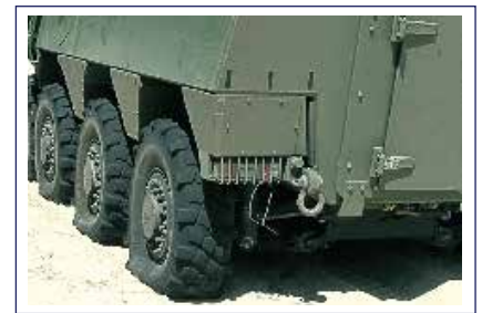
The beadlock function of VFI Runflat allows mobility during low pressure operation.
