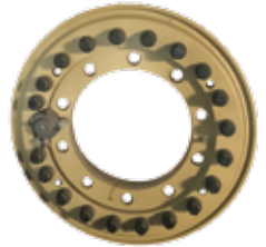
Hutchinson Aluminum Wheel w/ Integrated CTIS
