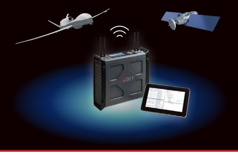
Trouble shooting tool for FDD/TDD LTE Field Test Record and store LTE signal by IQ format Real-time display of RRC/NAS messages Increase receiving gain by multi-units combination
