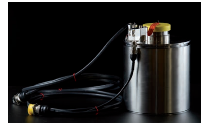
Connectors and cabling of a hydrogen burner.
