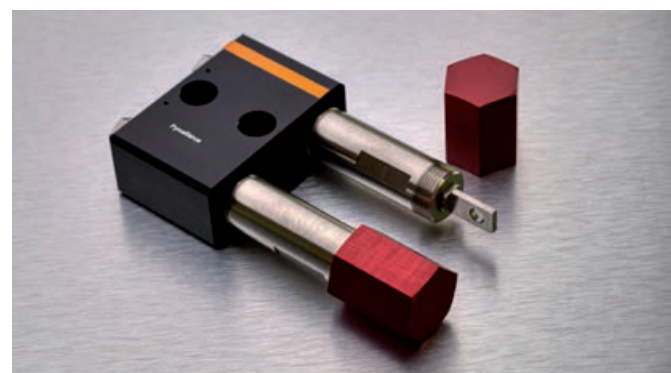
Canopy fracturing system: control unit (1/4).
